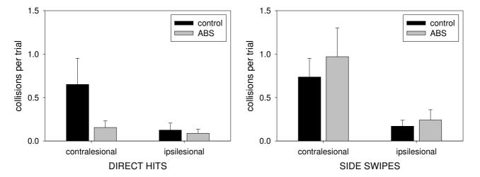
However, a reduction in direct hits for these patients was accompanied by an increase in side swipes (0.8 to 1.0 and 0.9 to 1.6). In some cases, side swipes were due to the chair avoiding a collision (due to ABS activation) on one side, only to generate a side swipe on the other. While, on balance, one would conclude that performance was improved by the ABS, these problems highlight the current weaknesses of the system, and inform challenges for the future with regards to further development.
